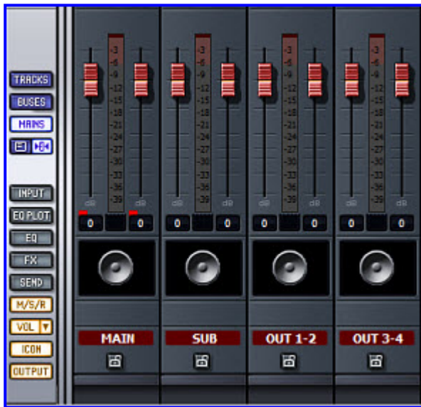
Figure 16: The MAIN button on the Surface gives you access to the VS-700R audio outputs.
