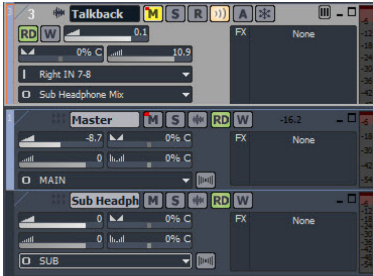
Figure 8: The talkback workaround utilizes an audio track, a headphone bus, and a master bus.
