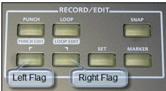
Figure 15: Use the Left and Right Flag buttons to clear a selection in Select mode.
